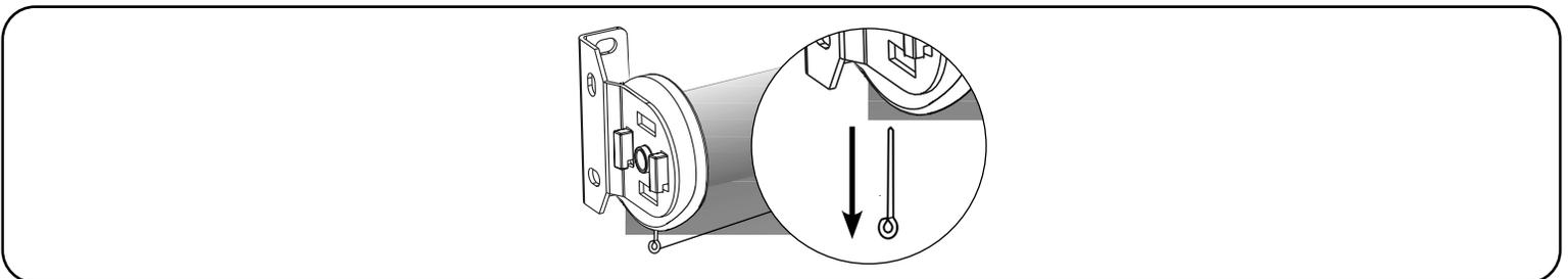
**Important:** Do not pull the lock pin until shade is securely assembled onto the brackets.
