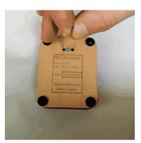
If the LED is still not blinking blue, clean any past WiFi network information stored by holding the "S" button for 10 seconds. The LED will blink blue faster after the "S" has been held for a full 10 seconds.
