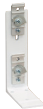
HDTB-B steel traverse bracket, double, can be used for single 6" return adjustable 5½"-6¼" front return adjustable 2½"-3½" back return 3¾"H x 1½"W backplate
