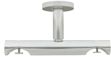
TFCMT118404 1 1/8" metal ceiling bracket, double 2 5/8" drop, 4 1/2" apart, 1 7/8" Dia ceiling plate
